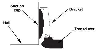
Portable transducer installed on boat transom.
